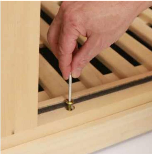
Install 4 furniture bolts through top and bottom of door frame using the allen key (included)
