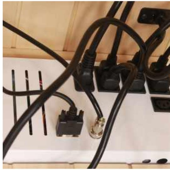
Feed the main power supply cord in through the hole in Back Wall and insert in power supply box.
