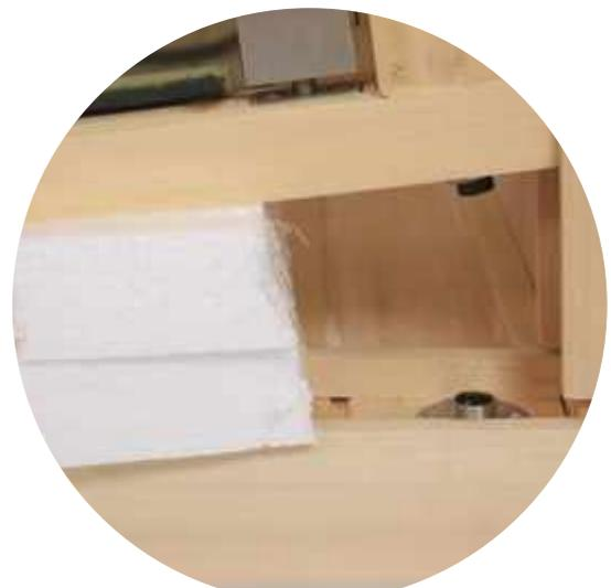
Connect door heater electrical lead to the floor base.
