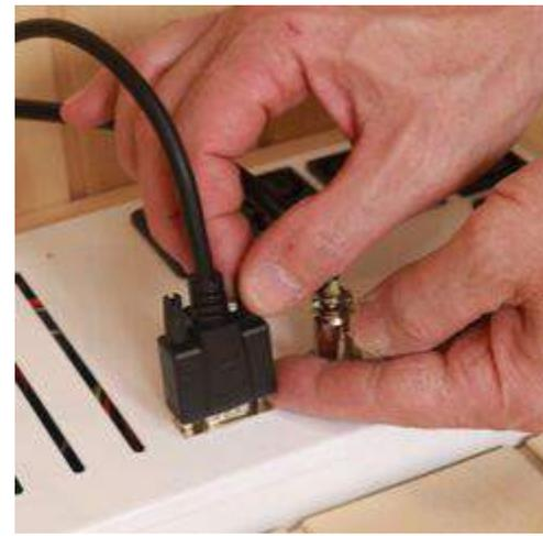
Attach the 'D-Sub' computer style connector as shown.
