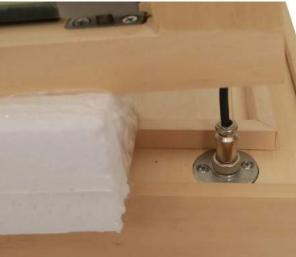
**Connect door heater electrical lead to the floor base.** Ensure hat the threaded cuff is fully screwed onto the floor base connector.
