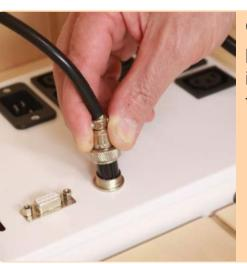
Connect the circular connector to power supply box. Align the groove in connector to properly insert. Thread the cuff of connector on fully
