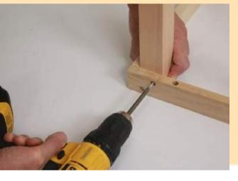
Ensure that the legs' ends are flush with the bottom edge of the frames
