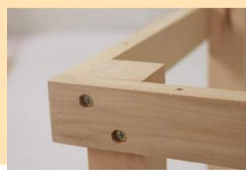
Attach the leg assembly to the bottom of the bench surface.Choose which surface of the bench you prefer to be the top and bottom.
