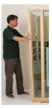
**Insert the Left Side Wall** into the channel of floor base while aligning the slot in Side Wall with edge of Front Wall glass panel.
