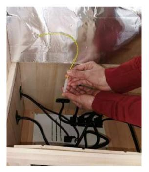
Connect the **grounding wire** from bottom side of Bench as shown
