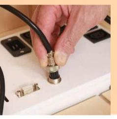
Connect the circular connector to power supply box. Align the groove in connector to properly insert. Thread the cuff of connector
