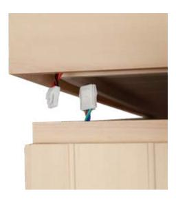
Connect the 12 V power line between the Side Wall and Roof.
