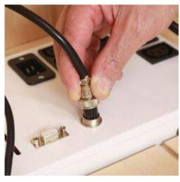
Connect the circular connector to Power Supply Box. Align the groove in connector to properly insert. Thread the cuff of the connector on fully.
